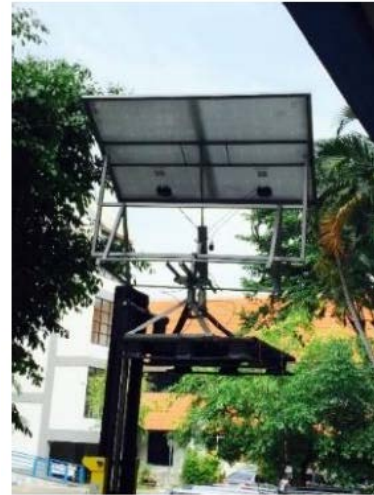
Figure 5. PV Position after Optimization with Dual Axis Solar Tracker based P&O method
