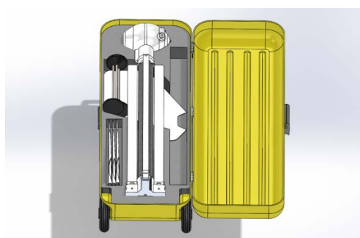
Figure 7 Wind turbine disassembled and packed into its case.
