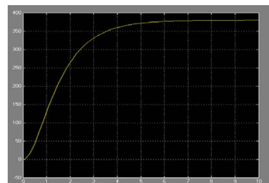
Figure 18 Power output using only wind, over first 10 seconds
