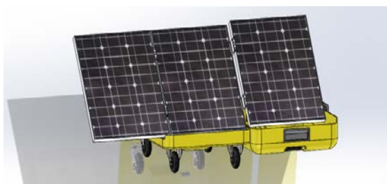
Figure 5 Front side of the solar array module, three 55W solar panels connected in parallel
