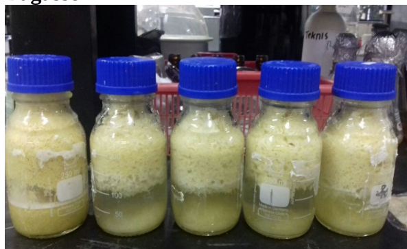
Figure 3. Pretreated sweet sorghum bagasse using NaOH hydrothermal with H_2O_2
